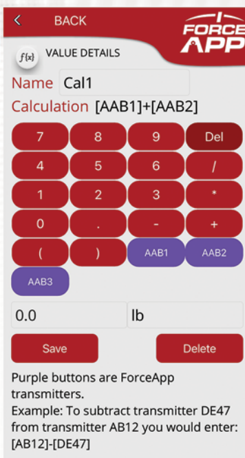
Calculated values—sum, subtract or add other calculations/ relations to view or datalog a derived value
